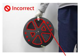
Do not hold the reel where the tape is exposed.
